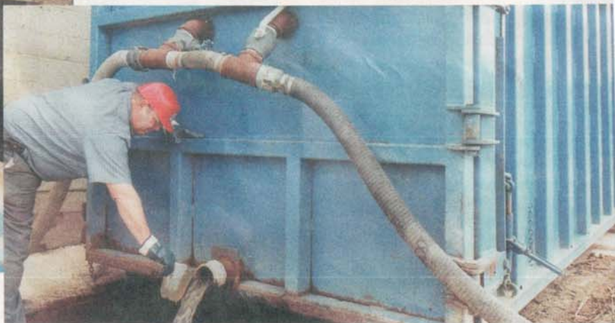
Tri-City dewateres septage in a DeTainer dewatering box supplied by Green Mountain Technologies. At the right, company president Gene Dube takes an effluent sample.
